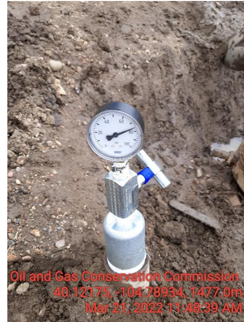
Photo 2 Casing pressure when opened
