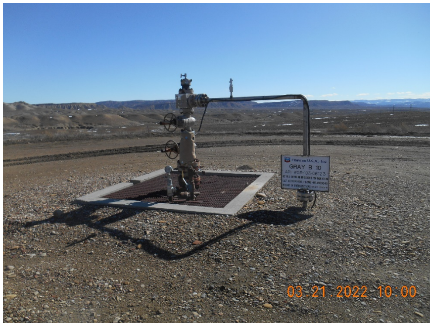
Injection wellhead
