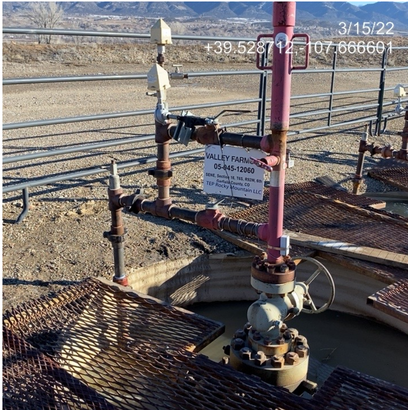
Photo 1. Photo taken from well API # 05-045-12060 facing north shows the well where a potential gas leak was observed in a previous inspection. Photo shows that water has been partially pumped from the cellar.
