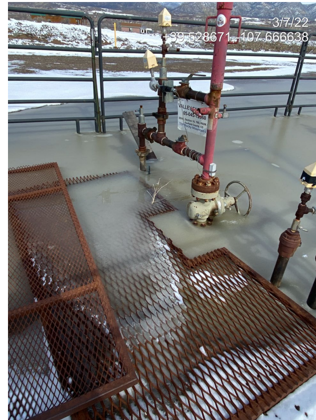
Photo 2. Photo taken from well API # 05-045-12060 during the previous inspection shows the cellar inundated with stormwater and bubbles in the water indicating a potential gas leak.
