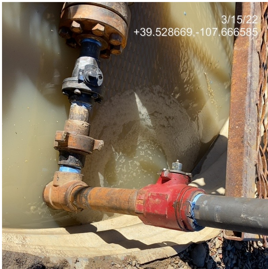
Photo 3. Photo taken from well API # 05-045-12060 shows the location of the bubbles from the previous inspection. Bubbles are no longer present. Photo shows new sealant tape on pipes indicating recent maintenance.
