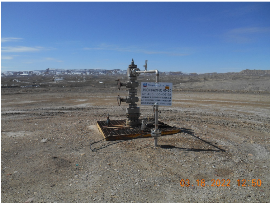
Injection wellhead
