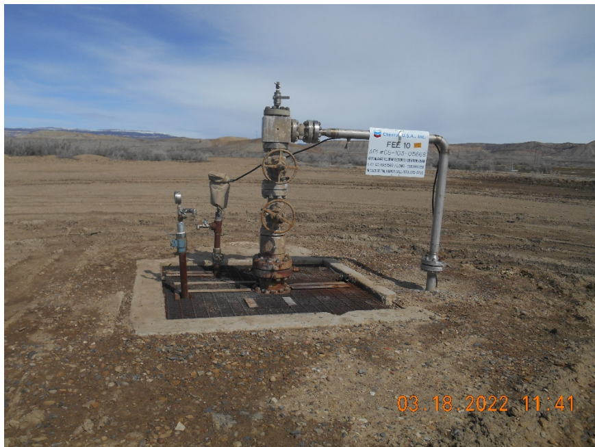
Injection wellhead
