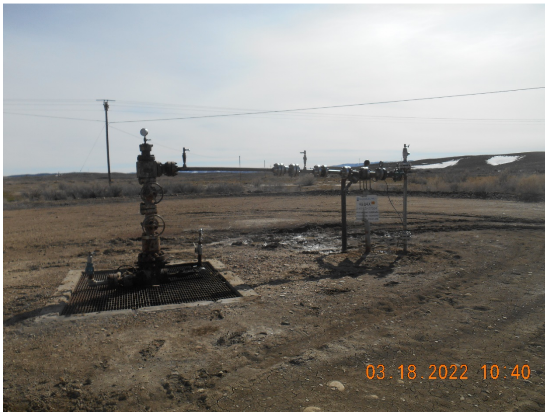
Injection wellhead
