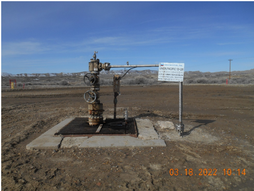
Injection wellhead
