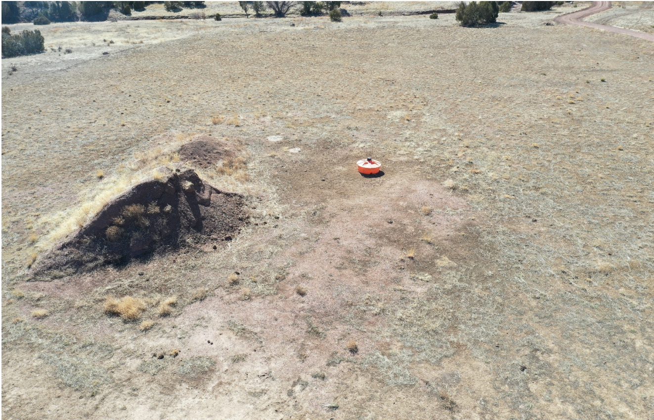
Photo 3. The gravel pile remains and should have been removed off the location to complete reclamation of this area.
