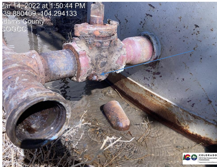
Pic 7 valve is leaking on middle steel tank
