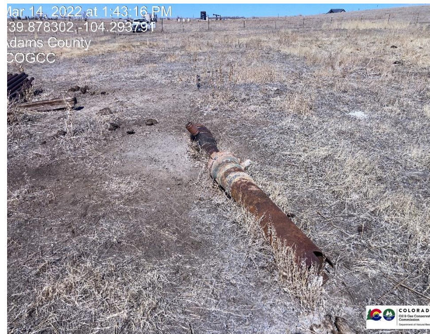
Pic 4 wellhead cut off on location.
