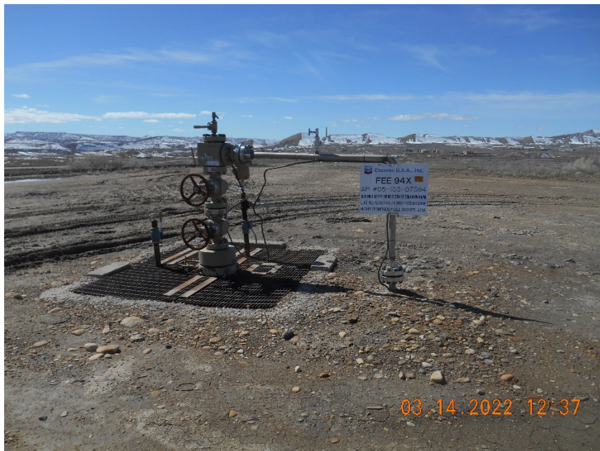
Injection wellhead
