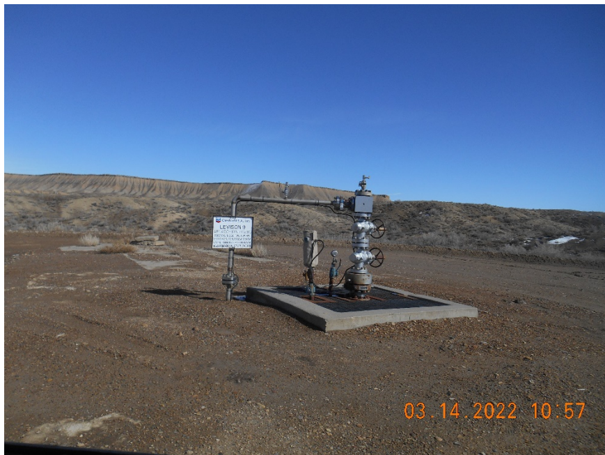
Injection wellhead
