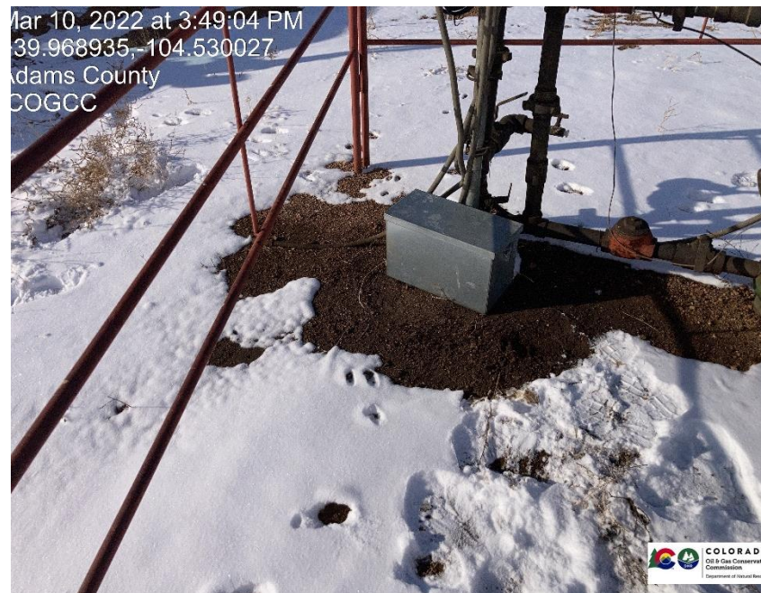
Possible flowline leak by wellhead. Stained soil around flowline.
