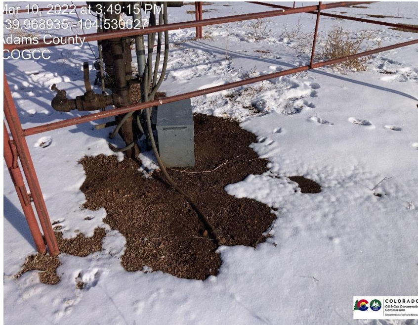
Pic 3 possible flowline leak by flowline going into ground.
