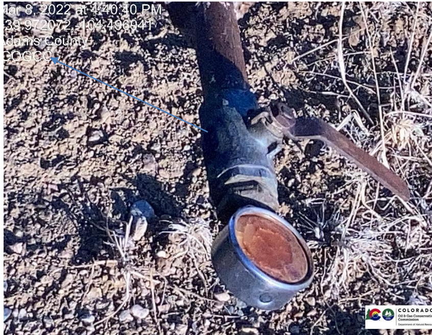
Pic 3 cracked ball valve. Venting gas.
