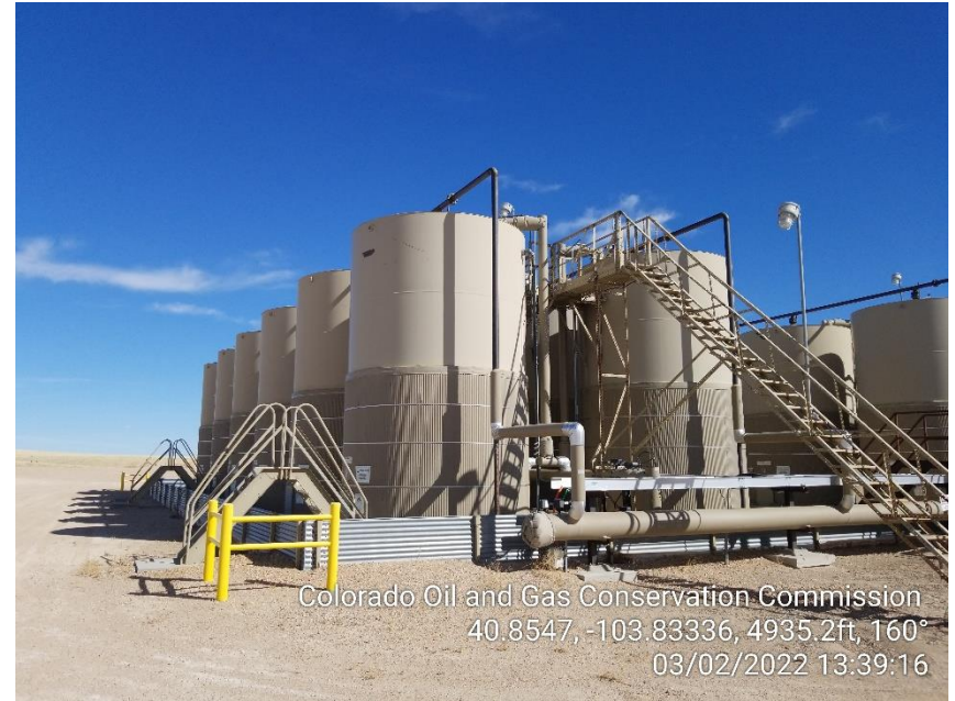
Photo 6 – Produced Water Tanks
