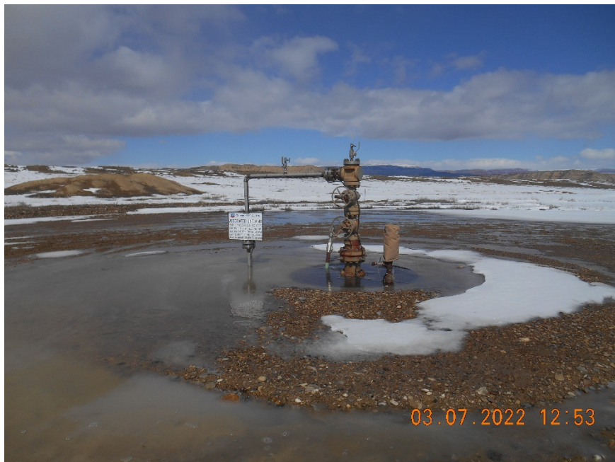
Injection wellhead
