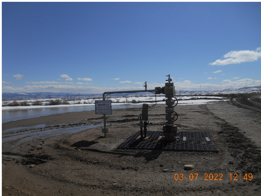
Injection wellhead
