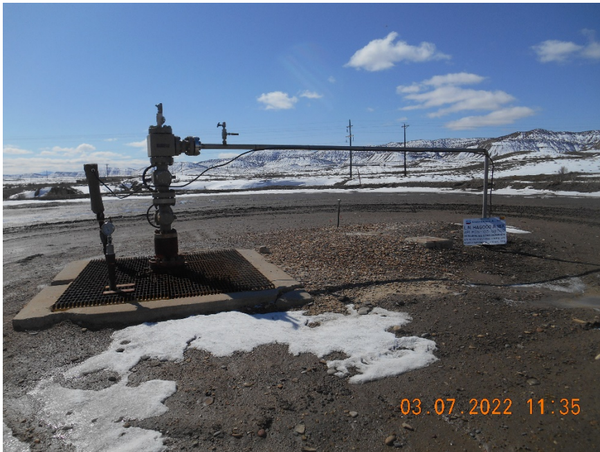
Injection wellhead
