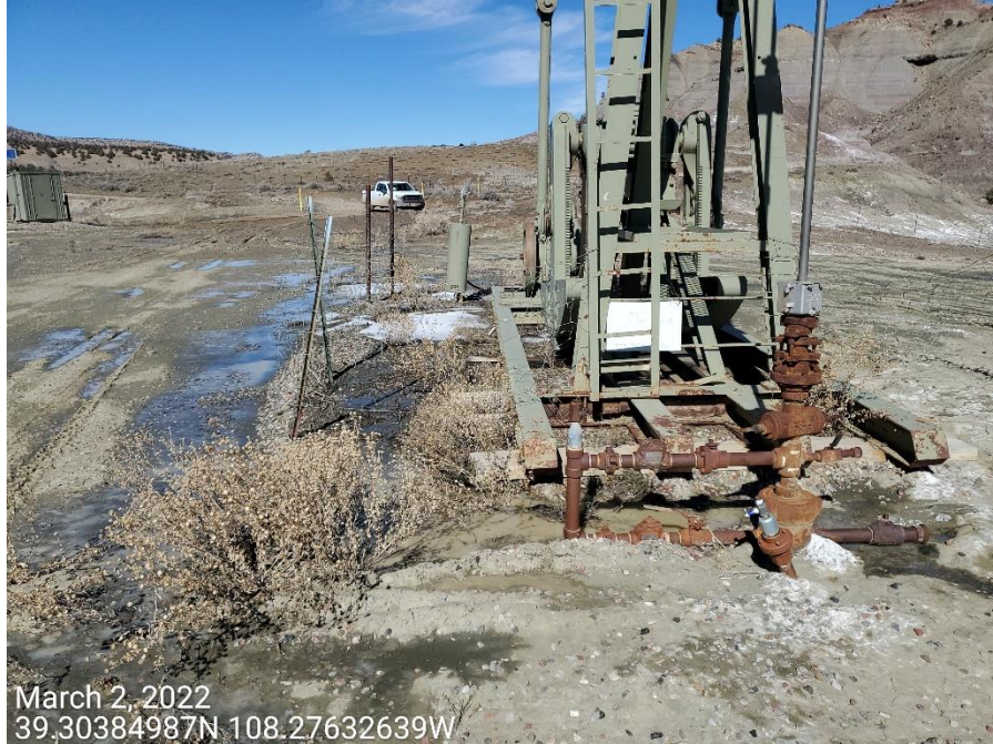
Photo 3: Photo shows vegetation/weeds have not been removed from around equipment.
