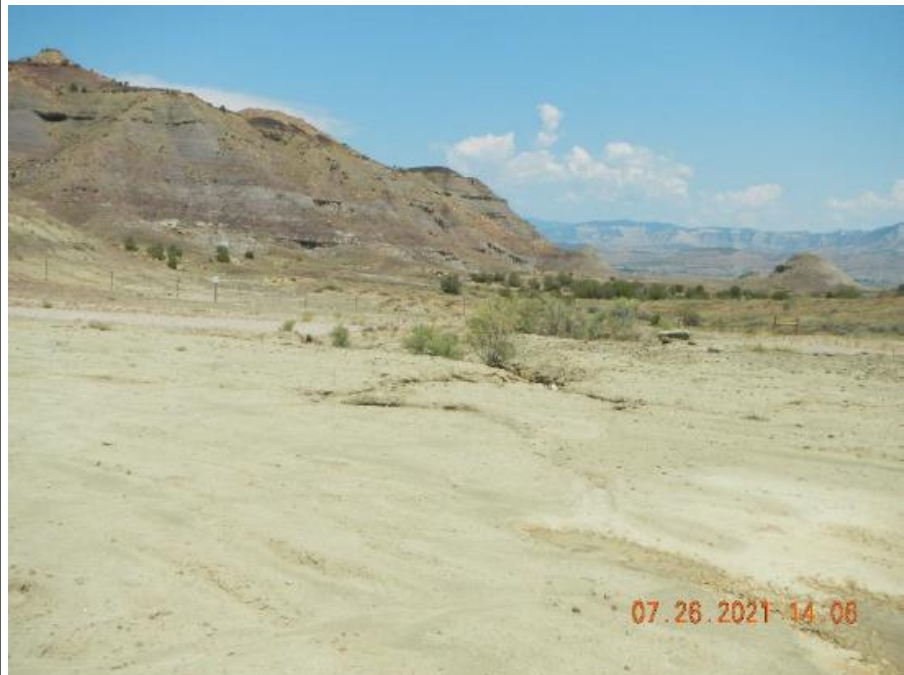
Photo 7: Photos taken from the east end of the Location, facing east. Photo left dated 7/26/2021; photos right 3/2/2022. Photo shows gully erosion degradation due to runoff from the location has continued since the previous inspection; control measures to manage runoff and minimize erosion degradation remain missing or insufficient on the Location.
