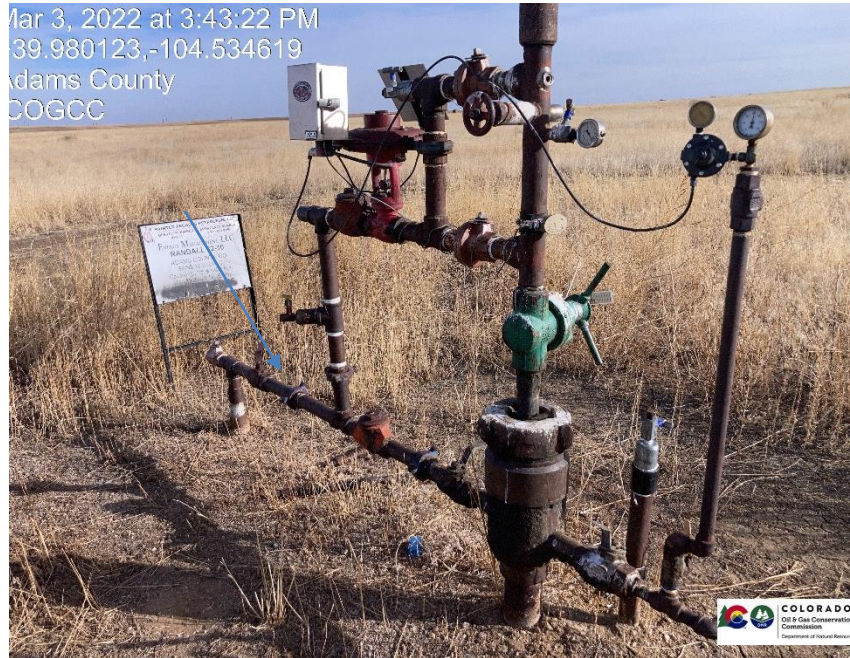
Pic 1 At time of inspection master valve, and casing valve were in open position. During inspection Master valve and casing valve were put in close position. Flowline valve is seized in the open position, casing valve, and tubing valve are both shut.
