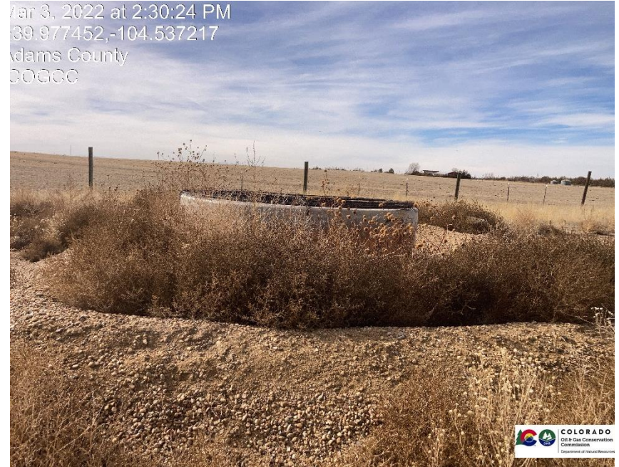
Pic 4 produced water open top tank, fluid present in tank.
