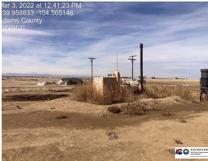
Pic 5 separator, ECD, abandoned gas meter run. Trash on location.
