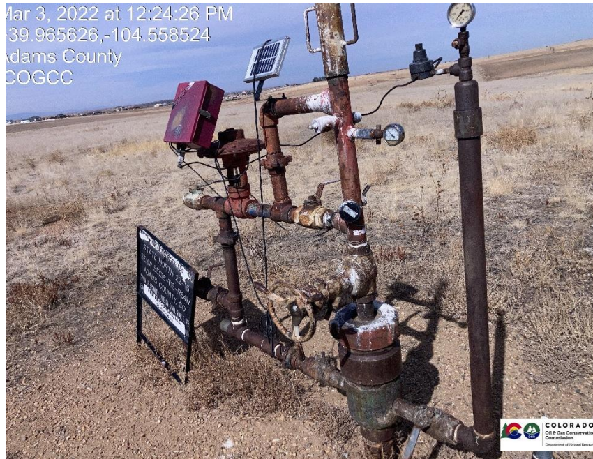
Pic 1 State Horth 22-16. At time of inspection master valve, and flow lines were in the open position. During inspection master valve and flowline valves were put in the close position.
