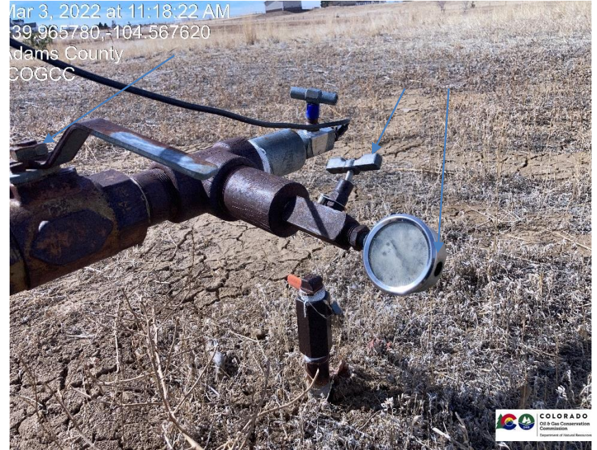
Pic 4 During inspection it was discovered that the wellhead was leaking gas out of the top of gauge pictured. Ball valve is seized in the slight open position, needle valve was open and shut during inspection. Needle valve is damaged and still has a slight leak of gas.
