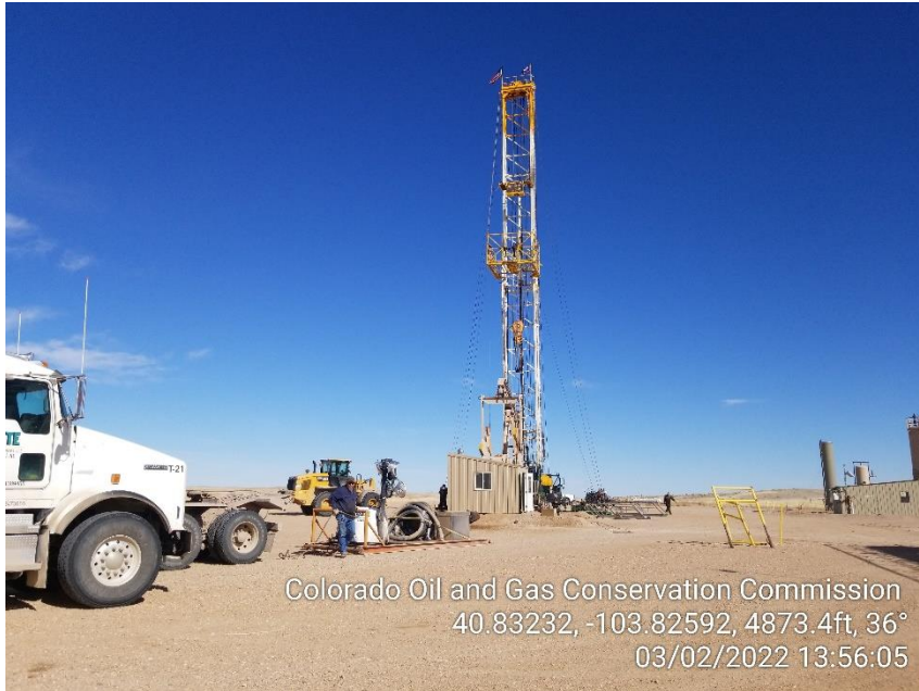
Photo 3 – Workover Rig in process of MIRU
