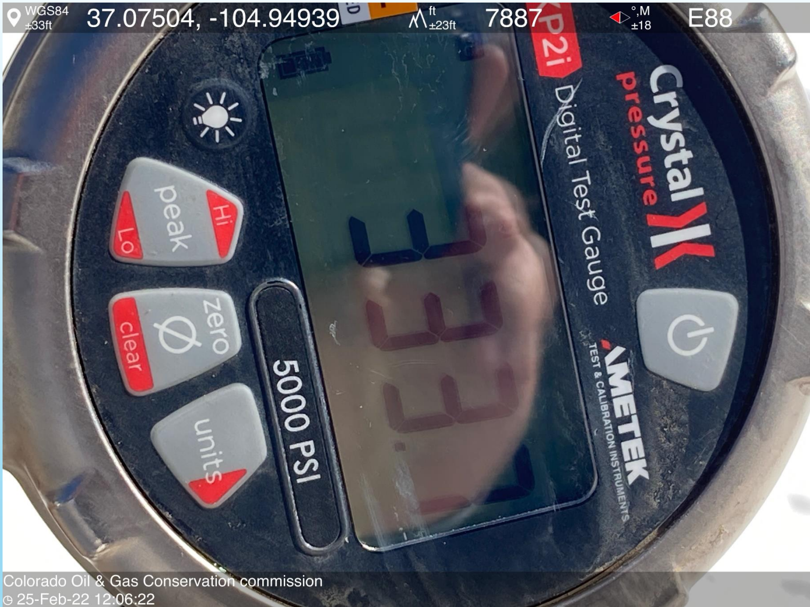
PHOTO 8: 15 MIN. FINAL MIT PSI 333.7, 2.5 PSI PRESSURE DROP DURING TEST, .9 PSI DROP DURING LAST 5 MIN.
