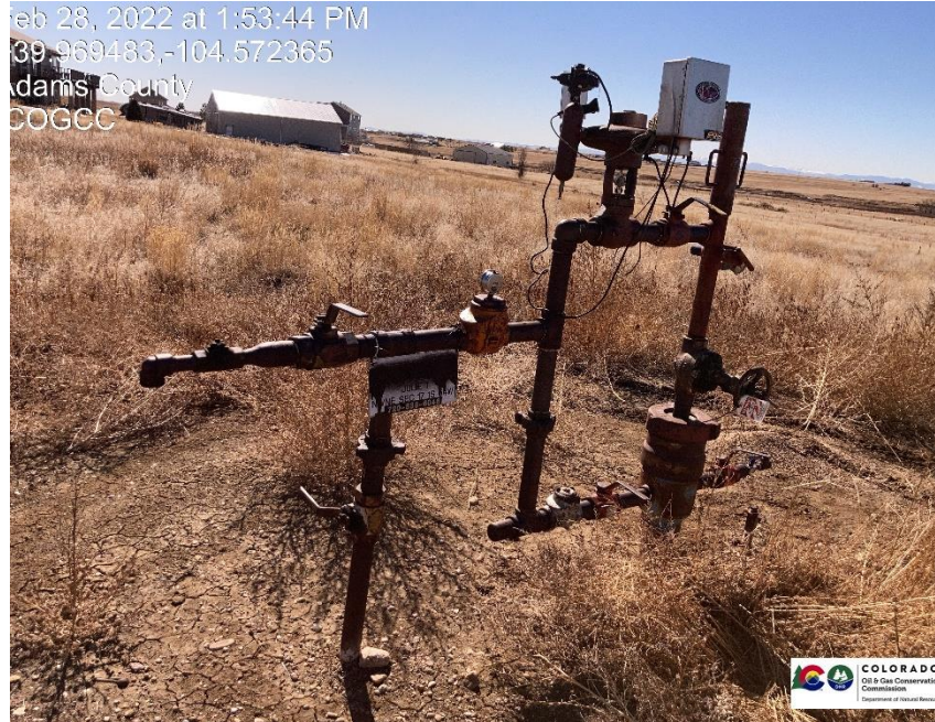
Pic 1 All ball valves were in close position at time of inspection. Master valve was seized in position, unable to determine if valve is open or shut. Bradenhead needle valve is shut.
