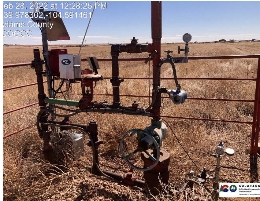
Pic 1 Master valve is free moving, and in the shut position. All casing, flowlines, and bradenhead valves are in the close position prior to inspection. LOTO is installed on master valve
