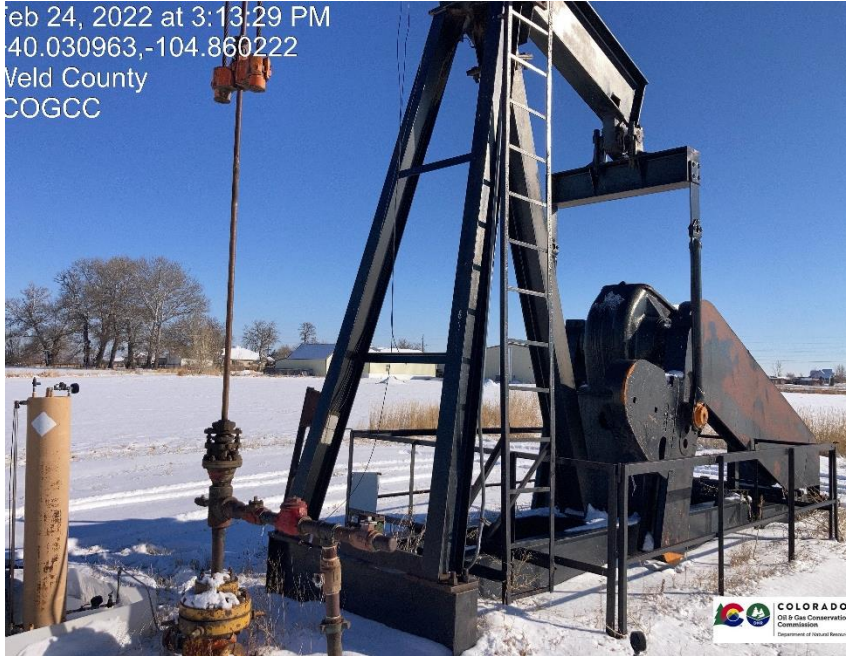
Pic 1 wellhead, electric equipment, pump jack.
