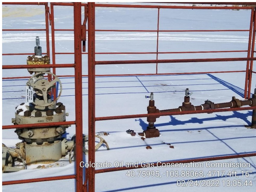
Photo 1 – TA Wellhead
