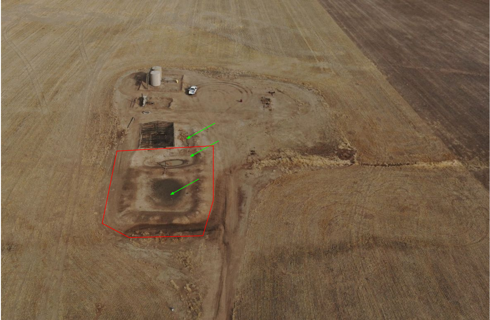
Photo 2. Operator is in process of closing 3 of the 4 pits per 900 series rules. Upon receiving final approval to close the pits, Operator shall further reduce the size of the location by returning 2 of the 3 pits back into crop production (red polygon).
