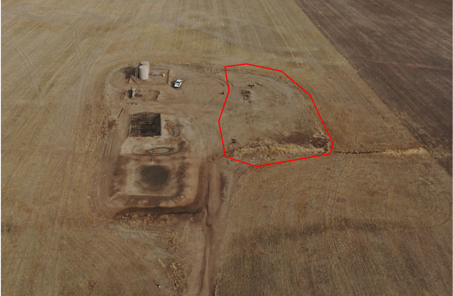
Photo 1. Drone aerial imagery illustrates the April #12-14 location. The photo illustrates the Operator has failed to complete final reclamation activities for the well location portion of the location (red polygon).
