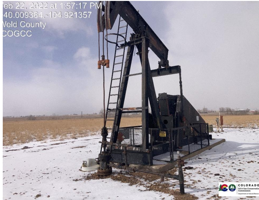
Pic 1 Pump Jack, wellhead.
