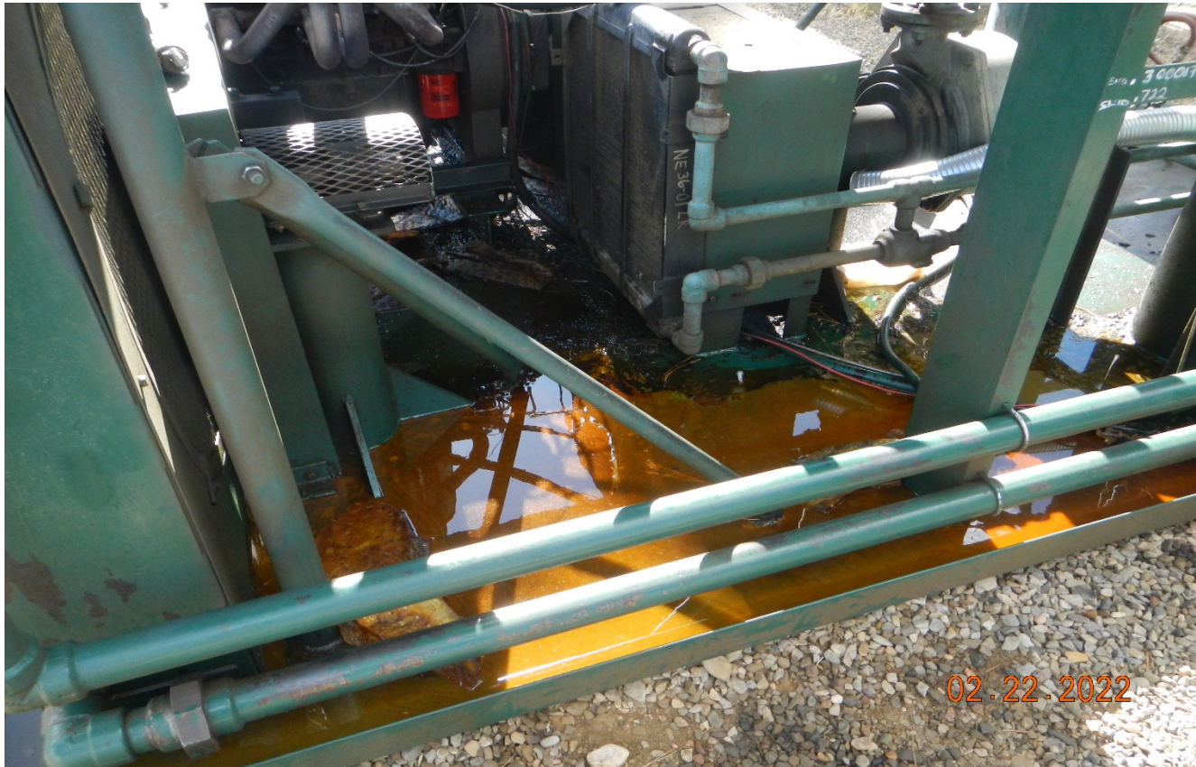
Photo 3. There is some oily rags and fluids on the engine skid.
