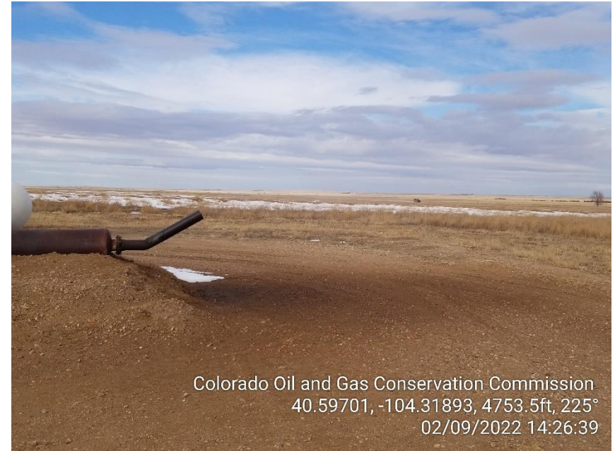
Photo 6 – Stained Soil at Exhaust
