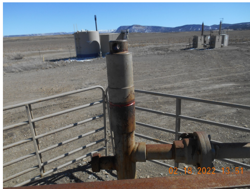
Leaking wellhead repaired. CA completed. API# 05-113-06131 ANDY'S MESA UNIT #41
