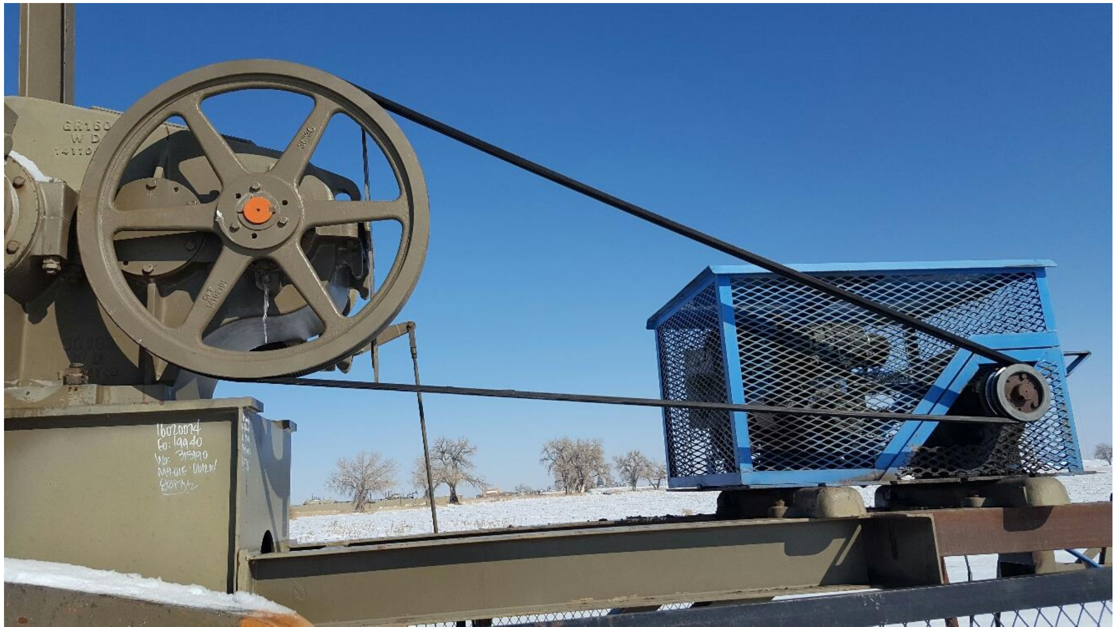
Figure #1 Belt has been re-installed.
