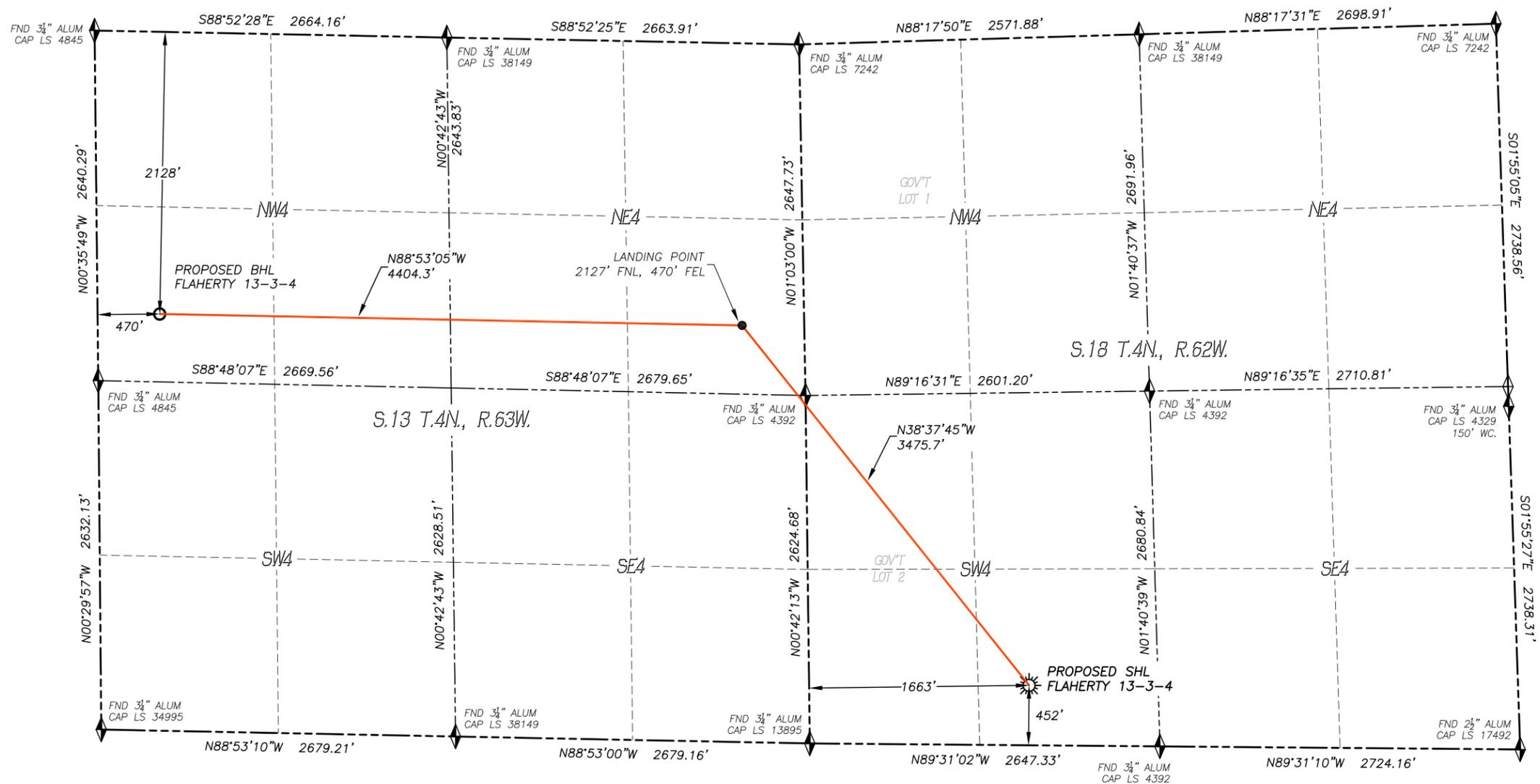
IN ACCORDANCE WITH A REQUEST FROM CONFLUENCE RESOURCES, DALEY LAND SURVEYING, INC. HAS DETERMINED THE SURFACE LOCATION OF THE FLAHERTY 13-3-4 WELL TO BE 452' FSL, 1663' FWL, AS MEASURED AT NINETY (90) DEGREES FROM THE SECTION LINES OF SECTION 18, TOWNSHIP 4 NORTH, RANGE 62 WEST AND THE BOTTOM HOLE LOCATION TO BE 2128' FNL, 470' FWL, AS MEASURED AT NINETY (90) DEGREES FROM THE SECTION LINES OF SECTION 13, TOWNSHIP 4 NORTH, RANGE 63 WEST, OF THE 6TH PRINCIPAL MERIDIAN, WELD COUNTY, COLORADO.
