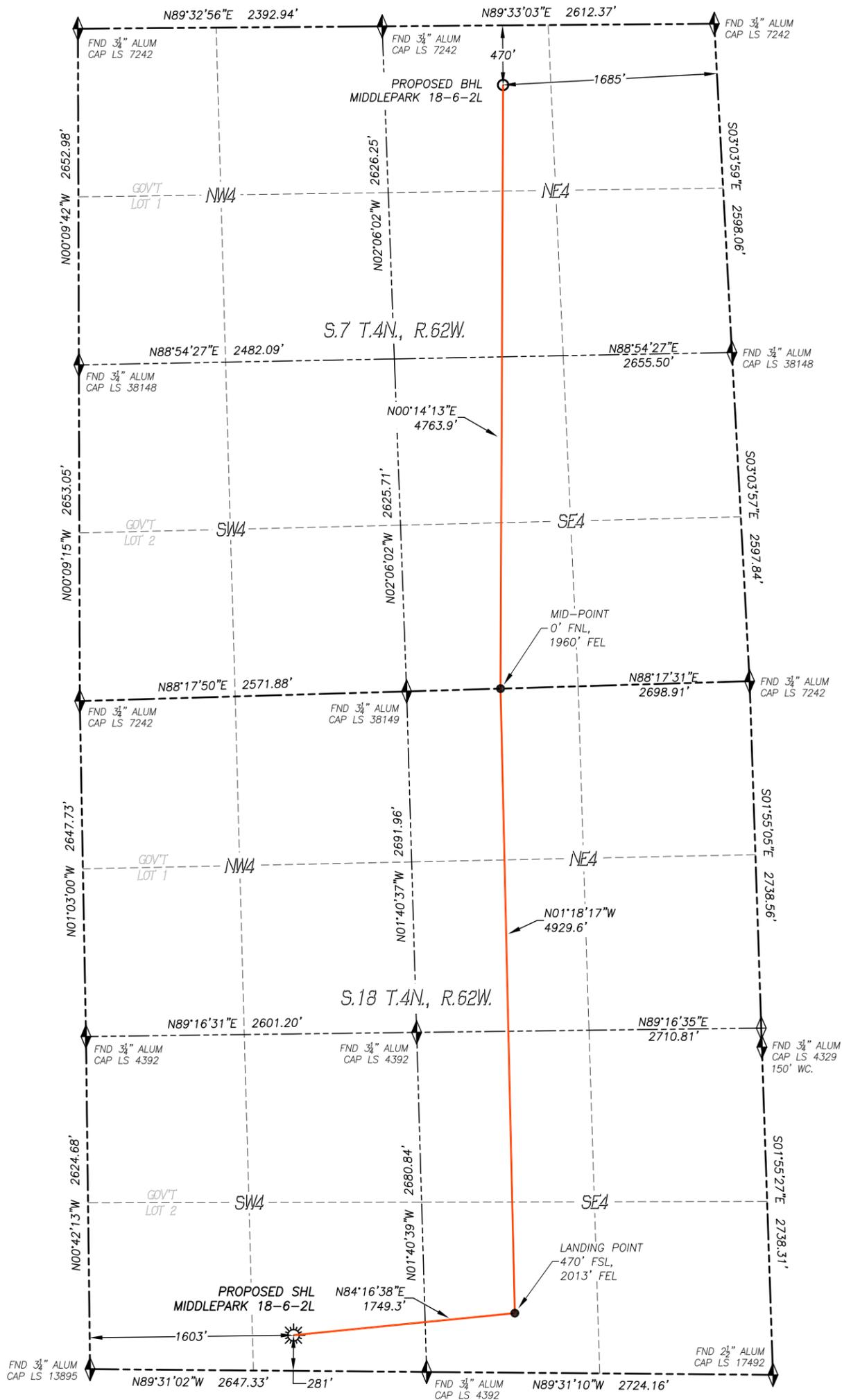
IN ACCORDANCE WITH A REQUEST FROM CONFLUENCE RESOURCES, DALEY LAND SURVEYING, INC. HAS DETERMINED THE SURFACE LOCATION OF THE MIDDLEPARK 18-6-2L WELL TO BE 281' FSL, 1603' FWL, AS MEASURED AT NINETY (90) DEGREES FROM THE SECTION LINES OF SECTION 18, TOWNSHIP 4 NORTH, RANGE 62 WEST, AND THE BOTTOM HOLE LOCATION TO BE 470' FNL, 1685' FEL, AS MEASURED AT NINETY (90) DEGREES FROM THE SECTION LINES OF SECTION 7, TOWNSHIP 4 NORTH, RANGE 62 WEST, OF THE 6TH PRINCIPAL MERIDIAN, WELD COUNTY, COLORADO.
