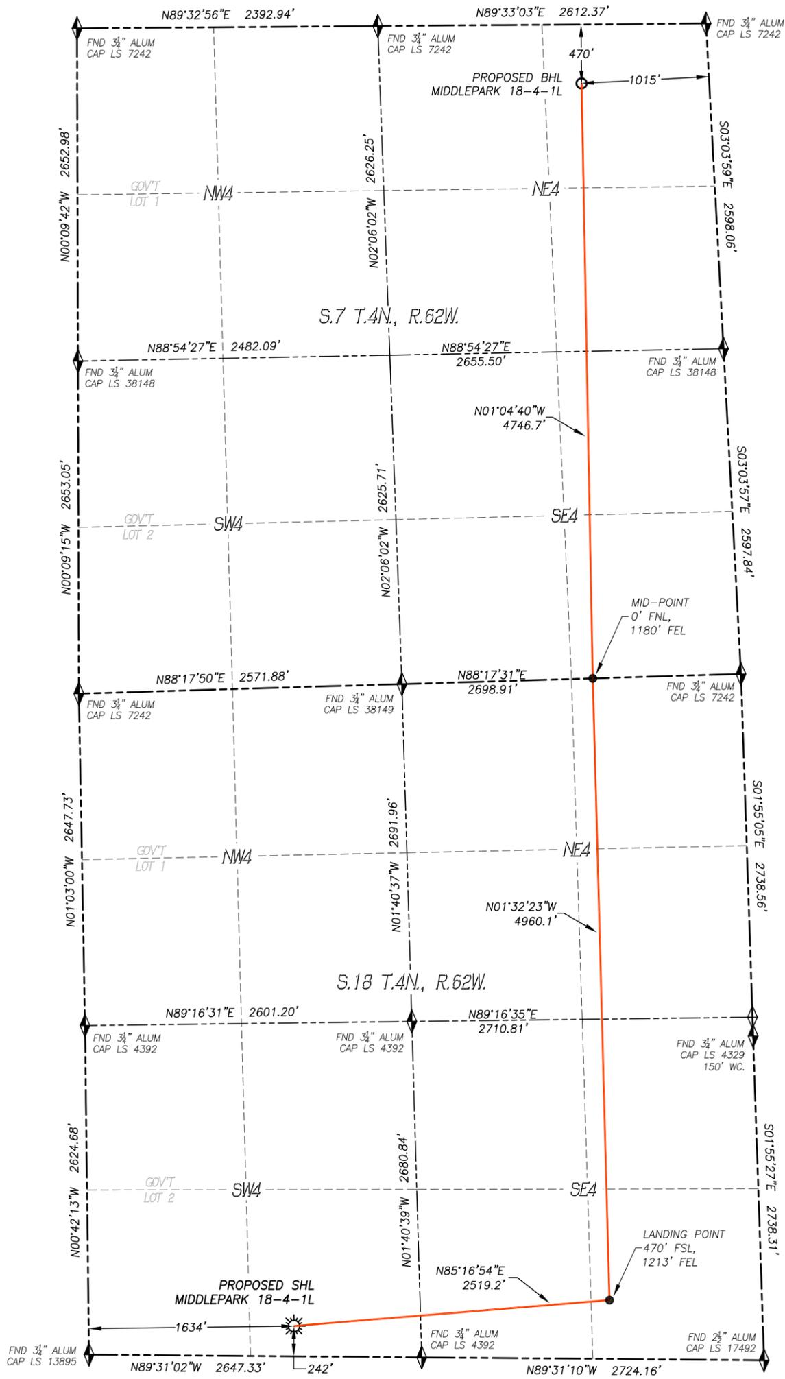
IN ACCORDANCE WITH A REQUEST FROM CONFLUENCE RESOURCES, DALEY LAND SURVEYING, INC. HAS DETERMINED THE SURFACE LOCATION OF THE MIDDLEPARK 18-4-1L WELL TO BE 242' FSL, 1634' FWL, AS MEASURED AT NINETY (90) DEGREES FROM THE SECTION LINES OF SECTION 18, TOWNSHIP 4 NORTH, RANGE 62 WEST, AND THE BOTTOM HOLE LOCATION TO BE 470' FNL, 1015' FEL, AS MEASURED AT NINETY (90) DEGREES FROM THE SECTION LINES OF SECTION 7, TOWNSHIP 4 NORTH, RANGE 62 WEST, OF THE 6TH PRINCIPAL MERIDIAN, WELD COUNTY, COLORADO.
