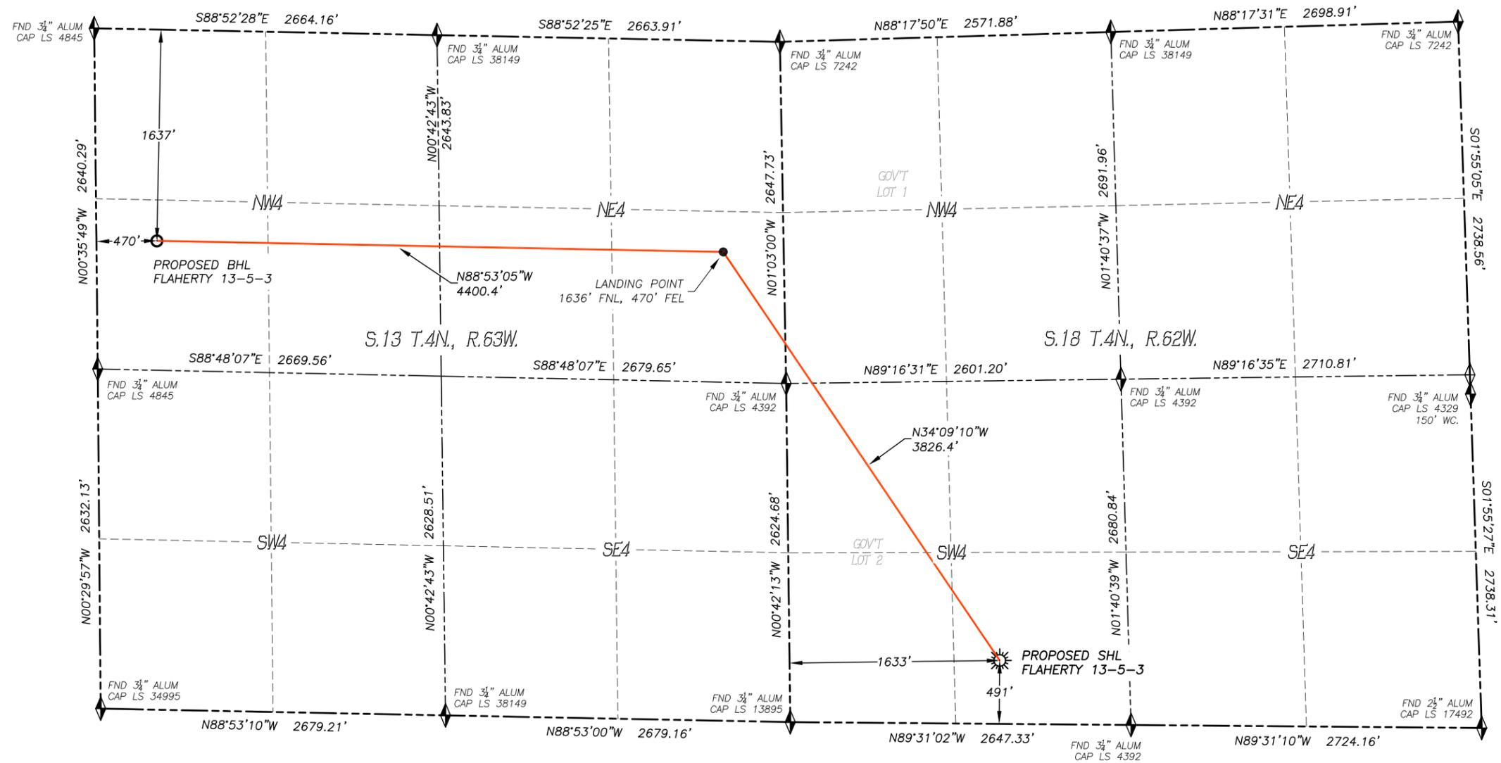
IN ACCORDANCE WITH A REQUEST FROM CONFLUENCE RESOURCES, DALEY LAND SURVEYING, INC. HAS DETERMINED THE SURFACE LOCATION OF THE FLAHERTY 13-5-3 WELL TO BE 491' FSL, 1633' FWL, AS MEASURED AT NINETY (90) DEGREES FROM THE SECTION LINES OF SECTION 18, TOWNSHIP 4 NORTH, RANGE 62 WEST AND THE BOTTOM HOLE LOCATION TO BE 1637' FNL, 470' FWL, AS MEASURED AT NINETY (90) DEGREES FROM THE SECTION LINES OF SECTION 13, TOWNSHIP 4 NORTH, RANGE 63 WEST, OF THE 6TH PRINCIPAL MERIDIAN, WELD COUNTY, COLORADO.
