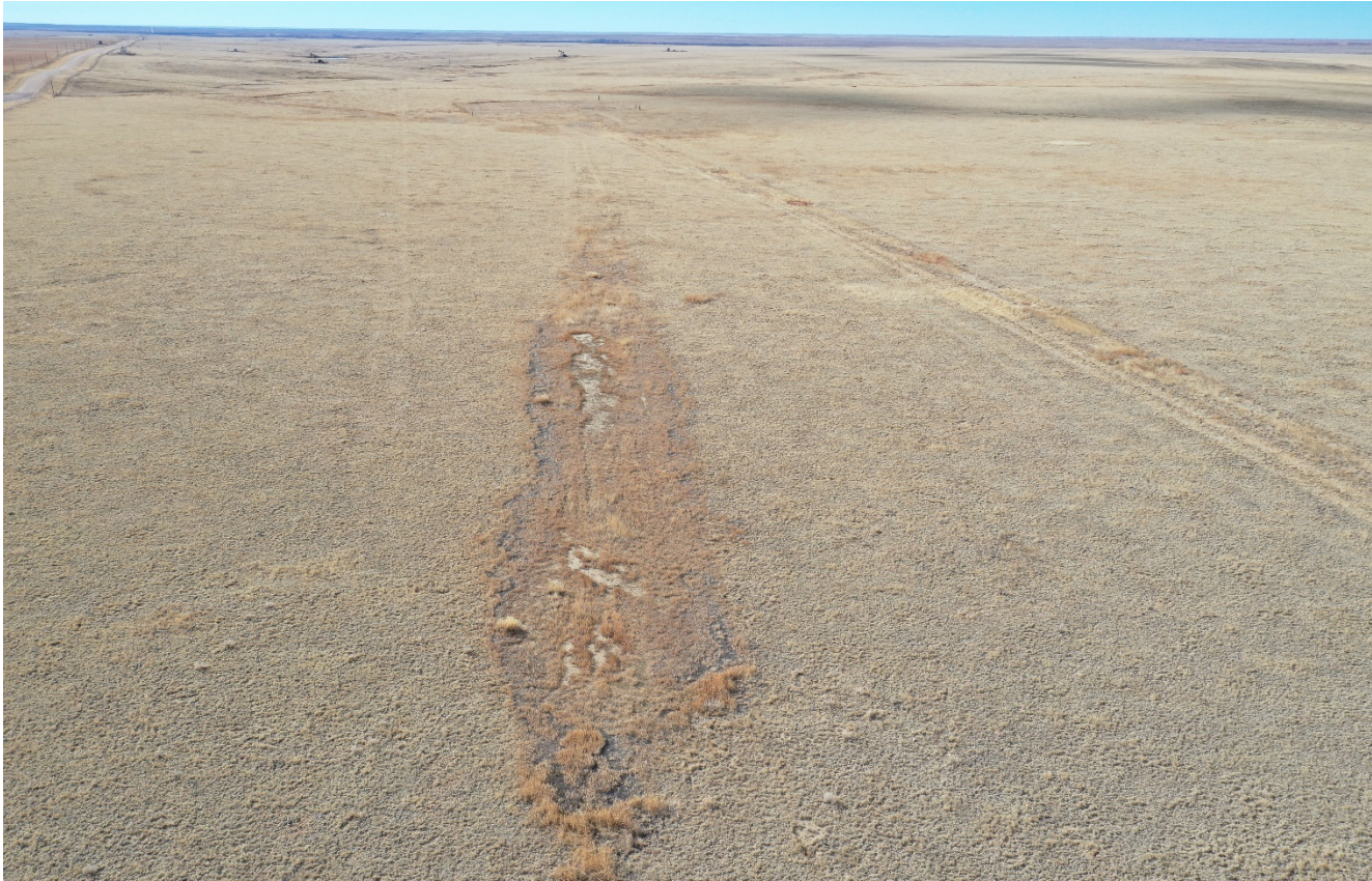
Photo 2. Drone aerial photo facing southwest along flowline area adjacent to the access road. It appears there was an impacted area along the flowline where vegetation is impacted.
