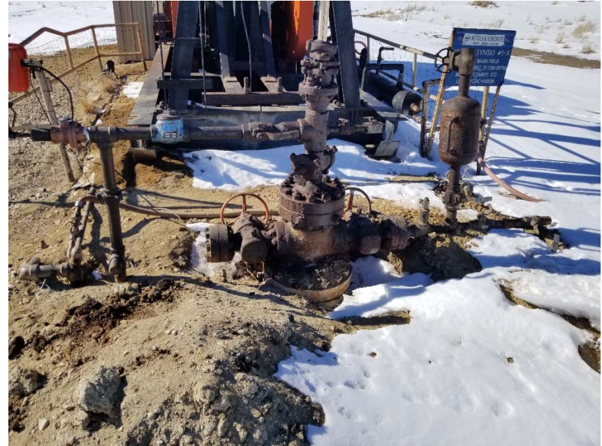
Photo 2. No bradenhead access apparent.
