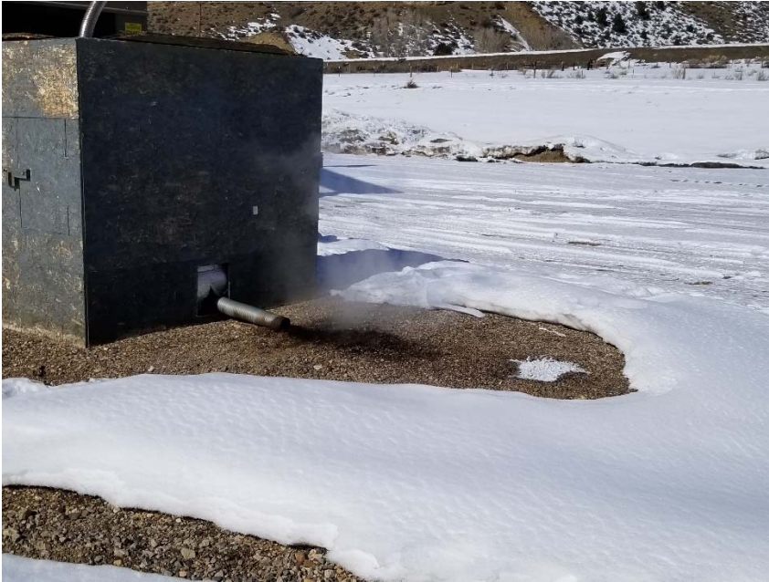
Photo 2. Stained soil at pump jack exhaust.
