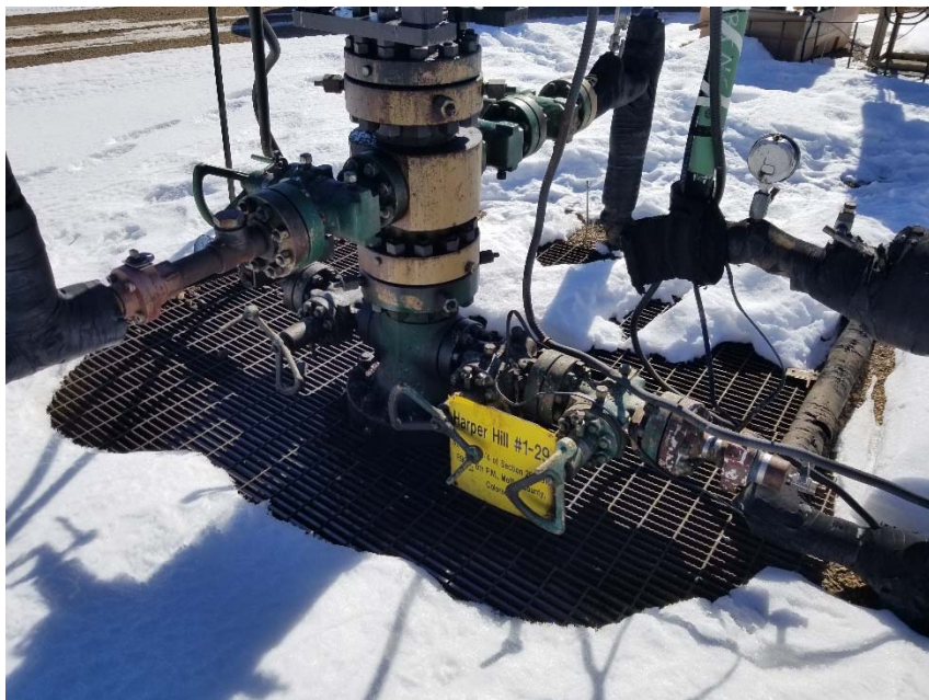
Photo 2. No bradenhead access apparent.
