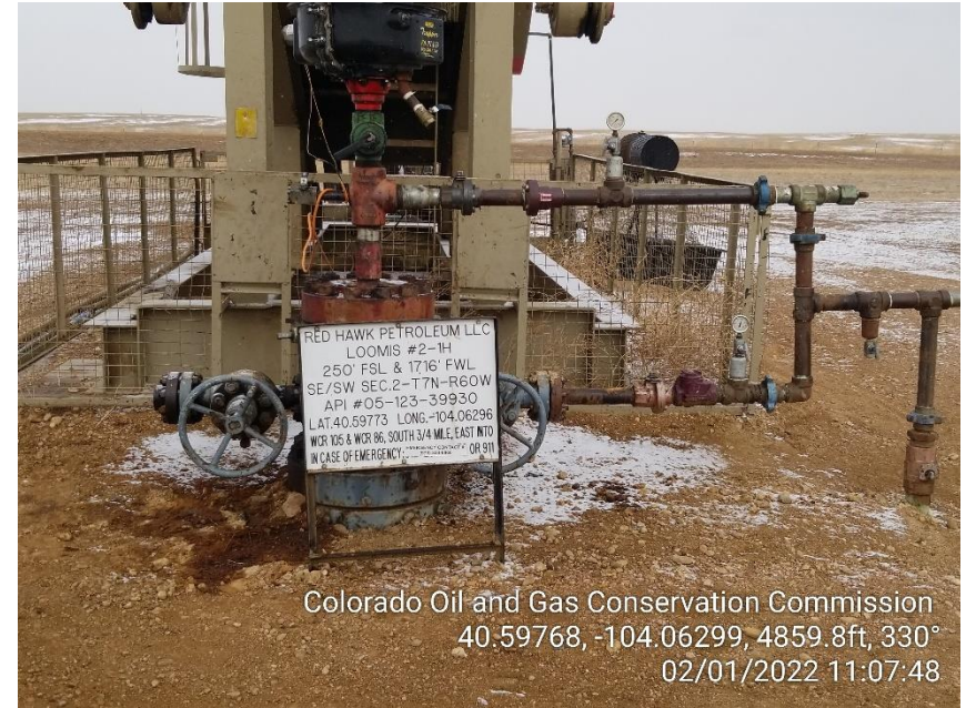
Photo 10 – 2-1H Wellhead – Stained Soil
