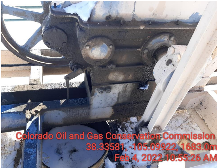
Photo 5 Mechanical issue gear box bearing leaking and creating stained soil under motor skid
