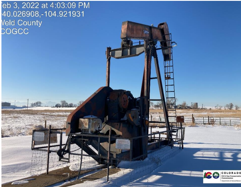
Pic 1 wellhead, electric equipment, pump jack.
