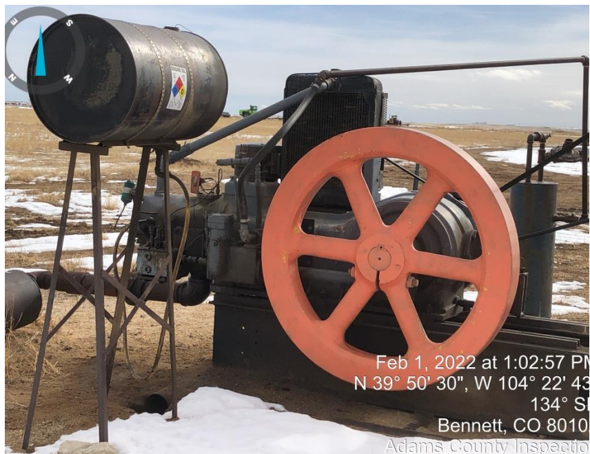
Photo#5 Corrective Action: No Secondary Containment under chemical tank. Repair or install berms or other secondary containment devices per Rule 603.o.
