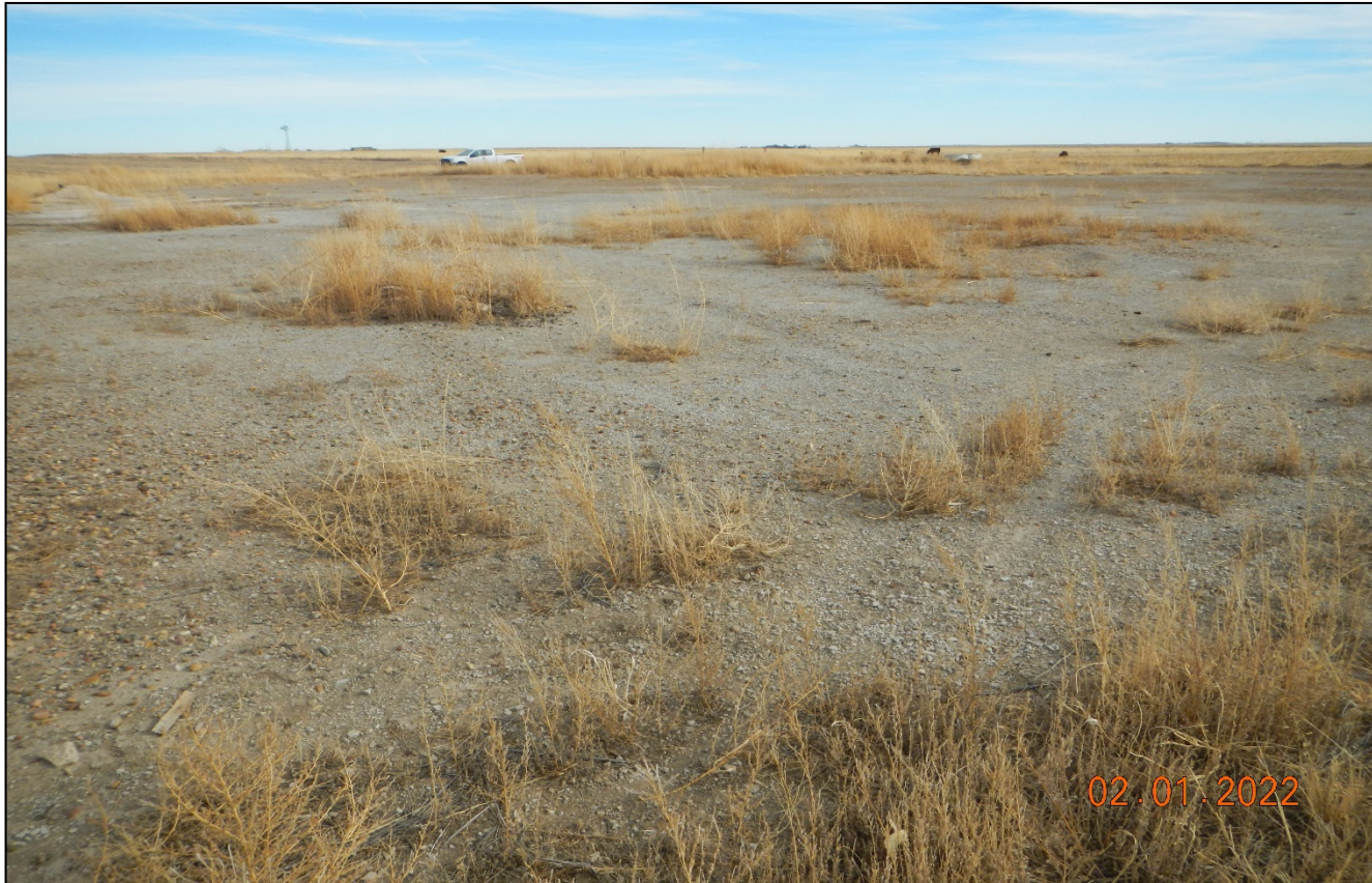
Photo 2. Facing southeast at the location. Soils are compacted and the location has not been reclaimed. Previous corrective actions were not performed. Soils must be decompacted by cross ripping to a depth of 18 inches.
