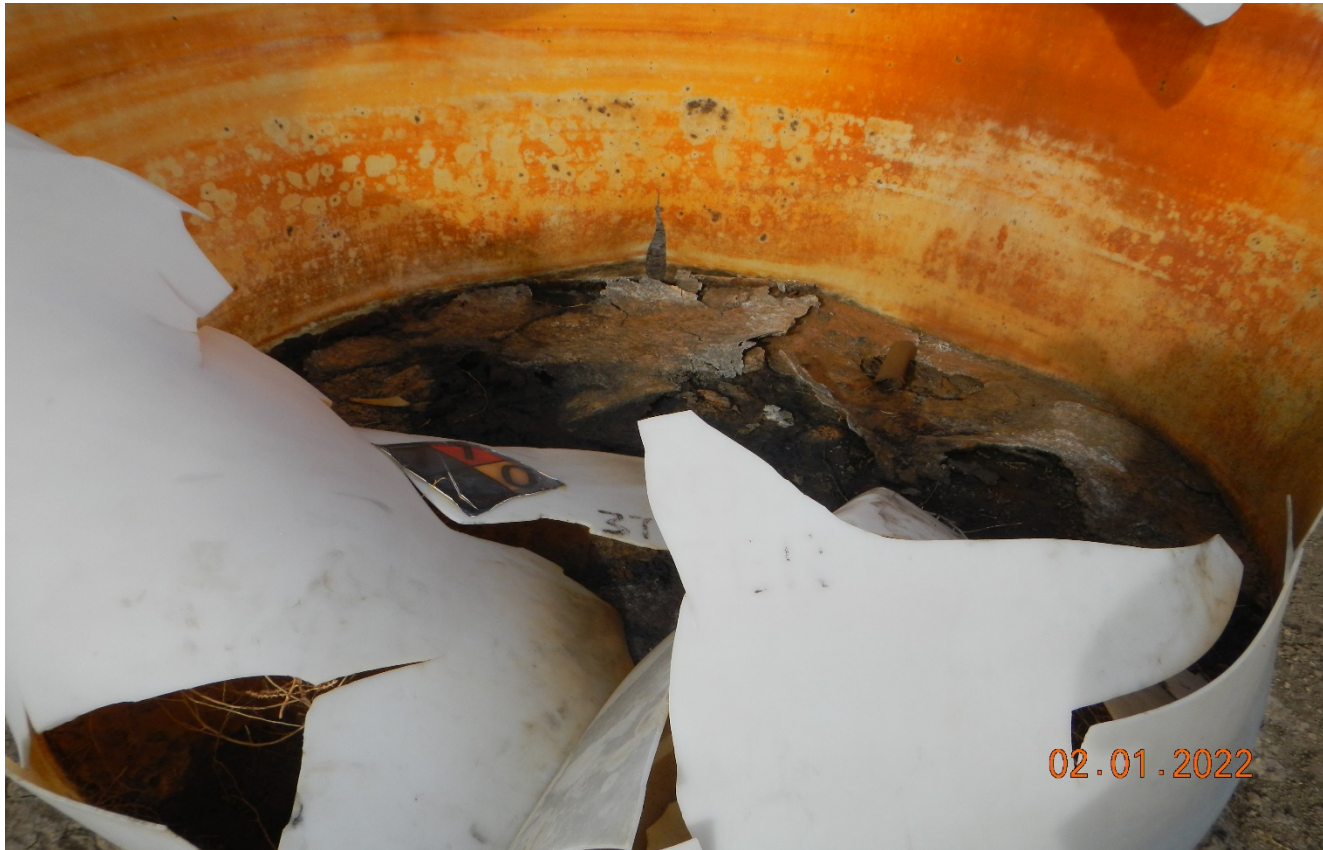
Photo 3. This photo shows the solidified oily substance inside the tank.
