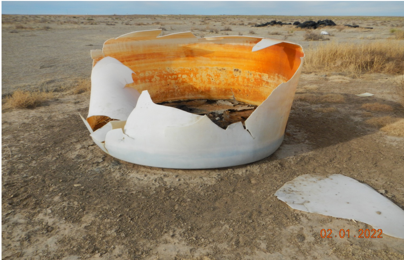
Photo 2. The tank on the location is busted apart and there is a solidified oily substance inside the tank which appears to have spilled out.
