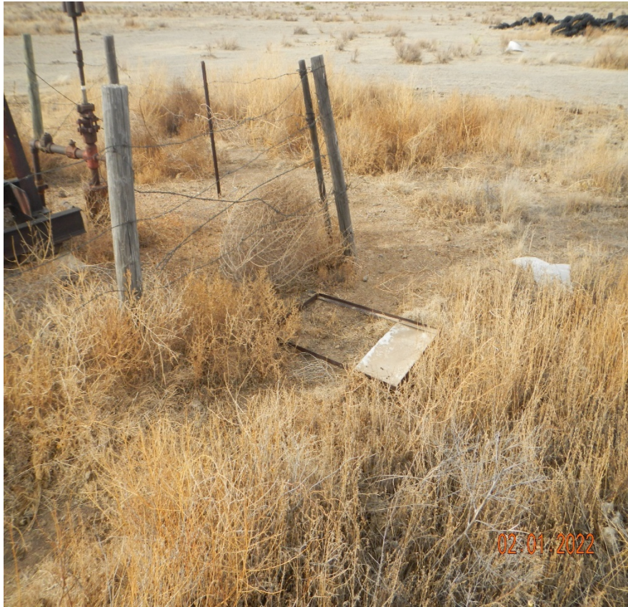
Photo 5. The well sign has fallen over and needs to be properly installed.
