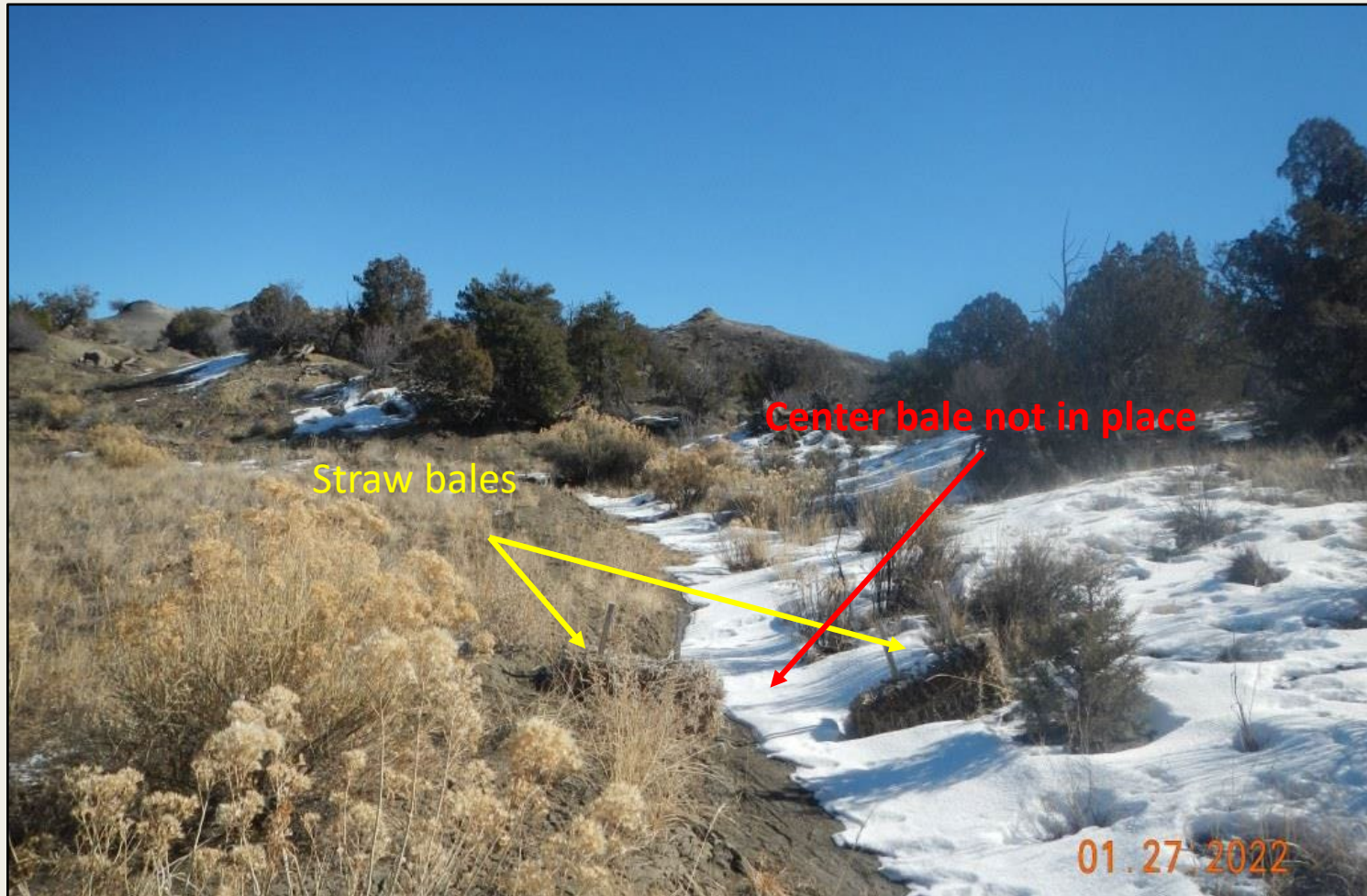
Photo 2. View of the southern project diversion facing eastward (upslope). Straw bails installed, are not an appropriate BMP to de-energize stormwater flows, additionally center straw bale is no longer in place.
