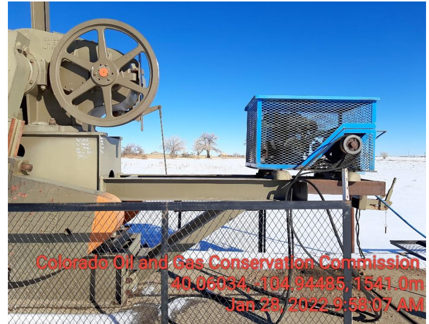
Photo 2 Mechanical issue Belts off motor
